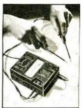
A "megger" cross-coil moving system is used in this meter (range—to 0.2-meg.). (1421)
